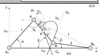
Fig. 2. Calculation of the coupler curves
