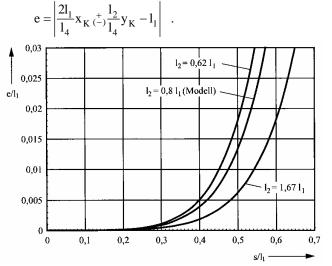
**Fig. 3.** Error e of the coupler curve  $k_K$  with respect to the line  $g_1$  depending on distance  $s = \overline{C_0 K}$ .
