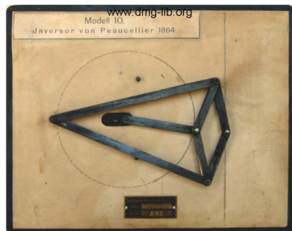
Fig. 10. Photo of a model of a Peaucellier–Lipkin invensor on which the metadata description in Figs. 11 to 14 is based on
