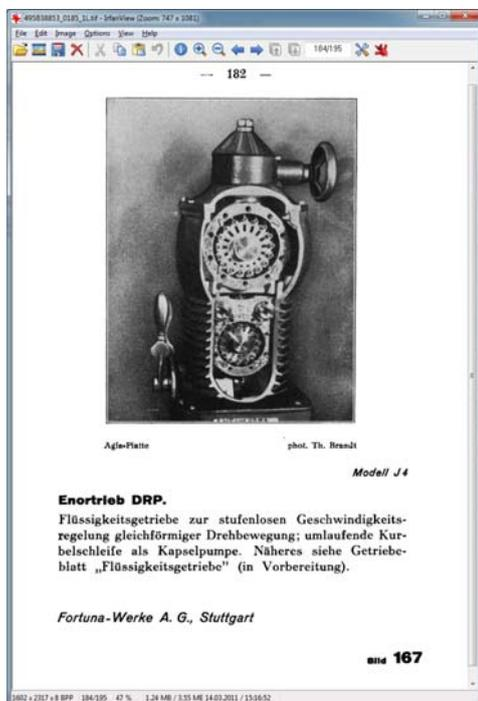
Figure B14 - ScanTailor colour mode setting: **Mixed mode** Quality of the photograph is much better. Output file size of TIFF-LZW is 1,24MB.
