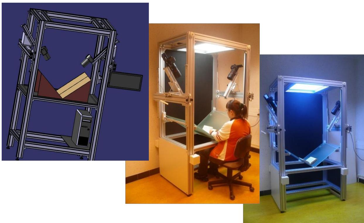
Figure 7. Self-made V-shape book scanner based on double EOS600D (18MPix each) developed by the French partner IFMA, CAD-Model and prototype
